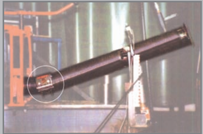
Angular Deflection: 20 degrees Pressure: 300 PSI
